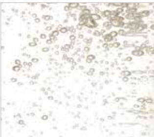
gas-to-liquid (GTL) air release: 15 seconds
